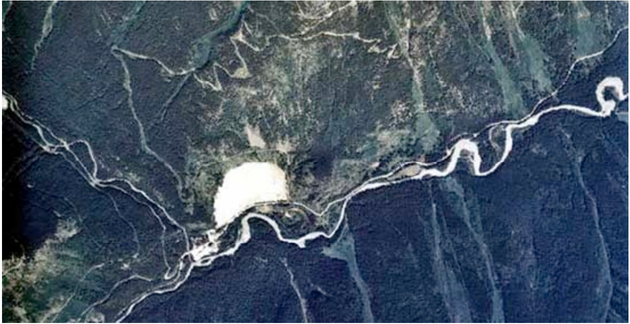
6. The junction of the Lower Jumbo Creek Valley with the Toby Creek drainage at the Mineral King Mine site. The mine's tailings are clearly visible (the big white area) and road alignments exist on both the north and south sides of the tailings. Toby Creek is the large light colored squiggly line that runs from the bottom left hand corner of the photograph to the upper right hand corner. Jumbo Creek intersects Toby Creek just before the mine tailings.
