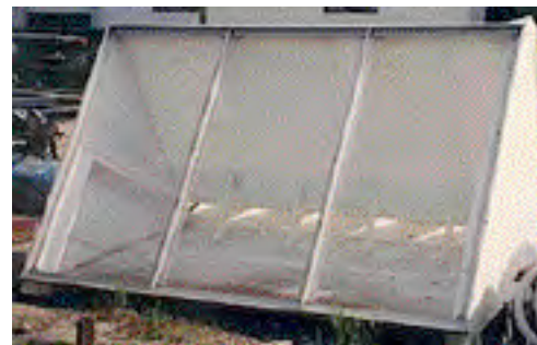
Bowen Island USBF clarifier
